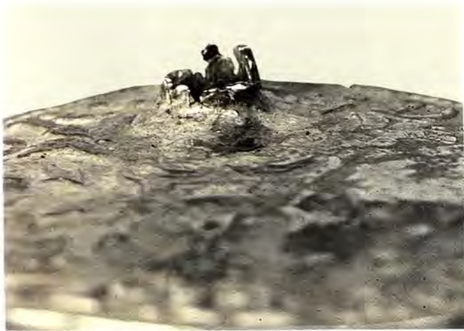
The sharp burrs resulting from punching in an unworked state.
